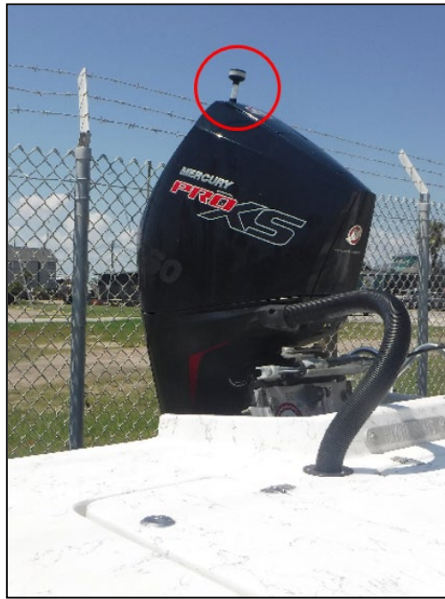
Figure 6. UPV 1 All-around white light close-up circled in red. Light was installed on outboard motor. (September 10, 2022/USCG)
