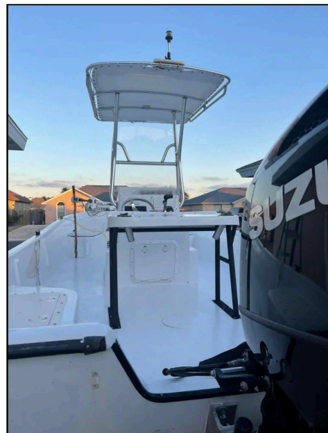
Figure 8. UPV 2 prior to collision with navigation lights intact, all-around white light location shown. (Unknown / Captain 2)
