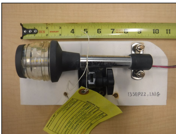
Figure 7. UPV 2 all-around white light, post-accident with ruler guide. (September 13, 2022 / USCG)
